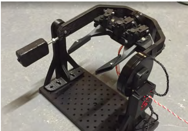
Figure 1. PV characterisation. Two-axis gimbal mounting system. Image source: Sensorica
