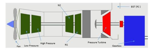
Figure 5.3: Gas Turbine Diagram [100]
