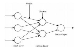
Figure 2.6: A Typical two-layer Artificial Neural Network [115]
