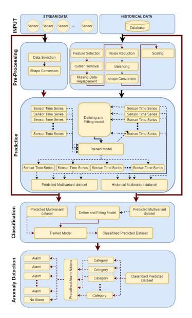
Figure 5.1: Activated Phases For Gas Turbine Analysis
