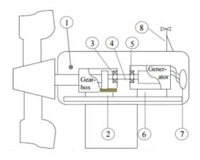
Figure 2.4: Schematic of Sensors in a wind turbine [125]
