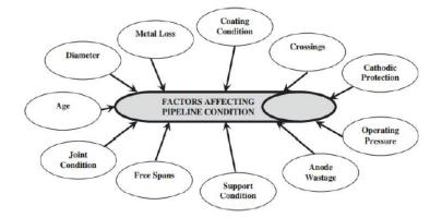
Figure 2.5: Factors affecting pipeline condition
