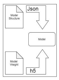
Figure 4.6: Load Model Weight and Structure
