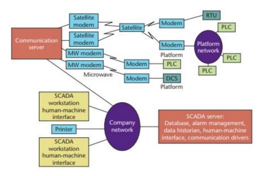
Figure 2.1: Supervisory, control, and data acquisition (SCADA) system for an oil platform
