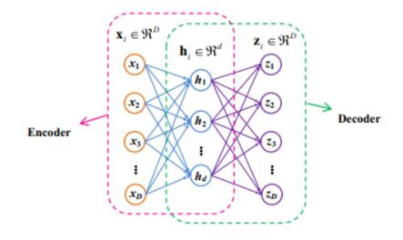
Figure 2.2: The Structure of an Autoencoder [132]
