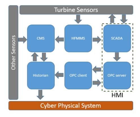
Figure 3.2: Data Monitoring Flow
