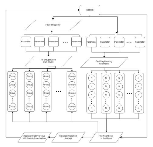
Figure 3.5: KNN Missing Replacement Procedure
