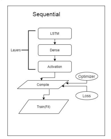
Figure 4.3: Compile and Fitting Diagram
