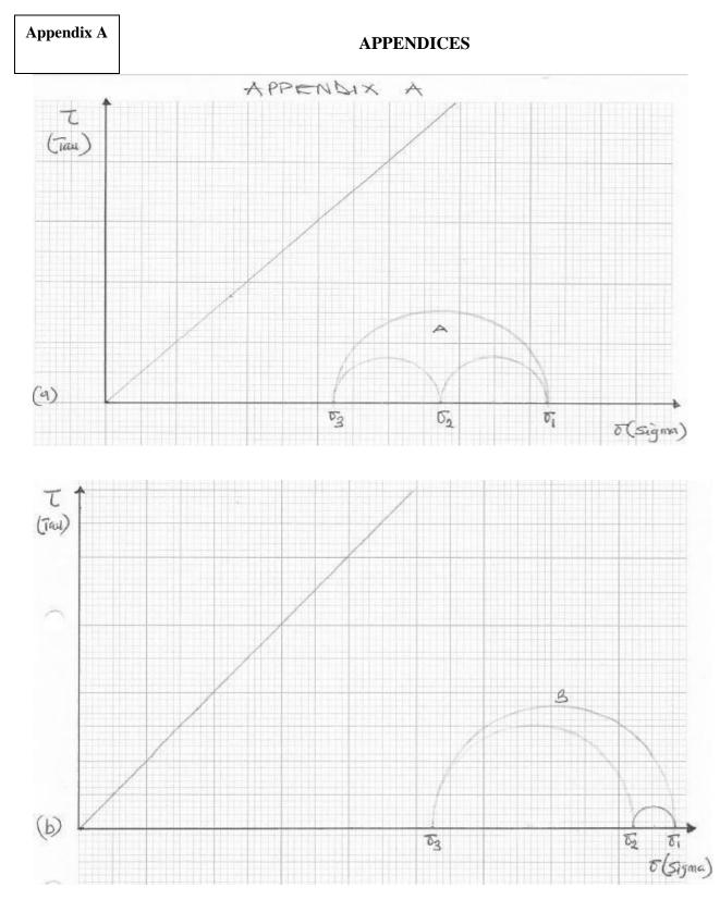
3D Mohr diagram construction for Wabi 05 stability of Wabi field for development design
