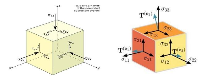
**Figure 2.7.** a) The normal and shear stress components on an infinitesimal cube. b) The stress tensor, a second- order tensor (Hudson and Harrison, 1997).
