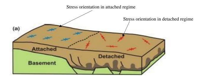
Figure 2.9. Schematic diagram of Attached and detached Stress regime (Bell, 1996; Tingay, 2009).
