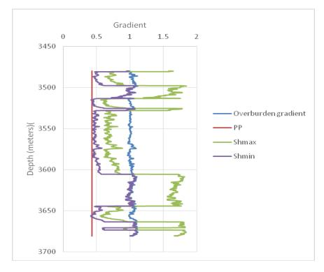
Figure 4.26. Pore pressure gradient/stress gradient for Wabi 11 reservoirs.
