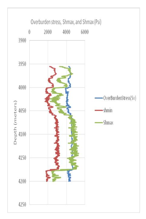
Figure 4.23b. Estimated stress profile model for Wabi 5 deep reservoir.
