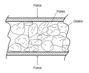
**Figure 2.11.** Show load sharing by pore pressure. Pore fluids support a portion of the total applied stress and only a portion of the total stress (effective stress) is carried by the rock.
