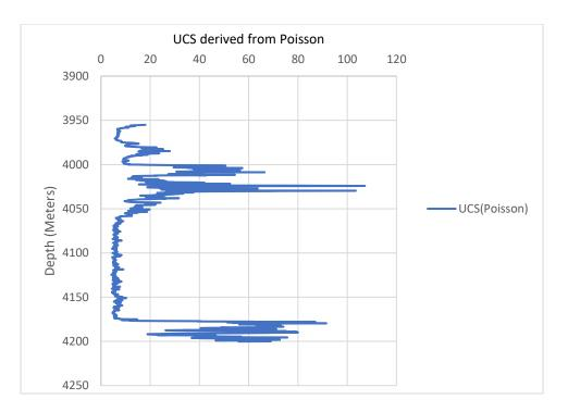
Figure 4.28b. UCS derived from Poisson's ratio for Wabi 5 Deep reservoir.
