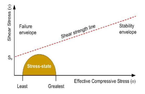
Figure 2.12. Mohr Coulomb failure envelope.
