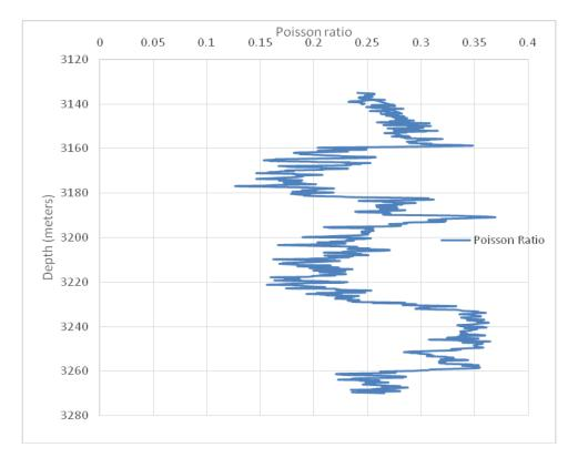
Figure 4.29a. Poisson's ratio in Wabi 5 for Shallow reservoir.
