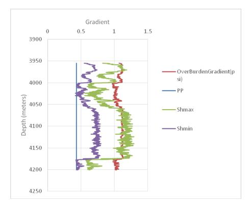
Figure 4.25b. Pore pressure gradient/stress gradient for Wabi 5 Deep reservoir.
