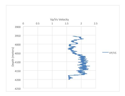
**Figure 4.5.**  $V_{P}/V_{S}$  profile for lithology delineation Wabi 5B reservoir
