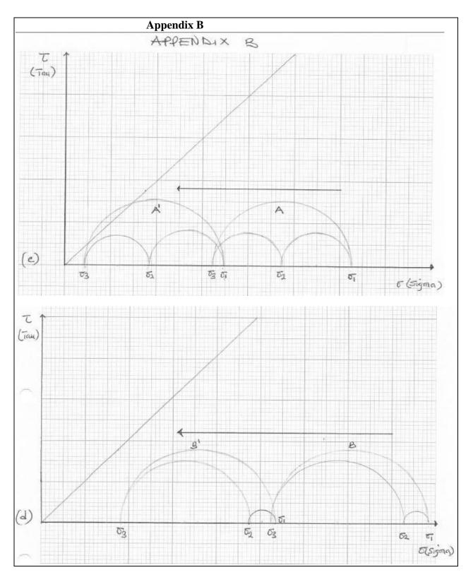
3D Mohr diagram construction for Wabi 05 showing movement of Mohr circle for injectivity scenarios Appendix C 1 2 3 4
