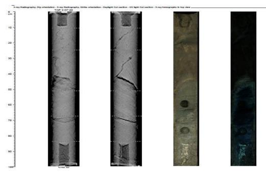
1&2): X-ray radiography showing dip and strike orientations,3.)Daylight cut and 4.) UV light cut section
