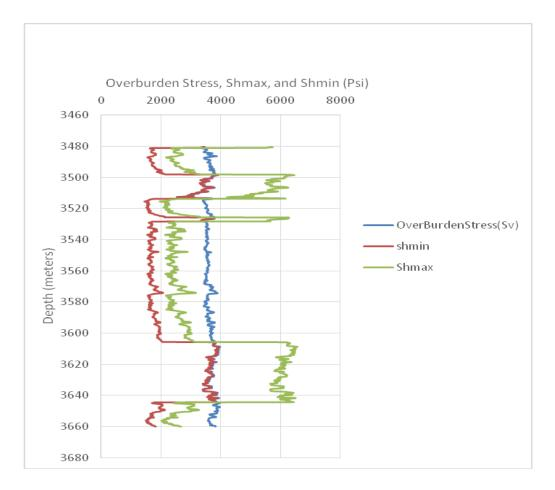
Figure 4.24. Estimated stress profile model for Wabi 11 reservoir.
