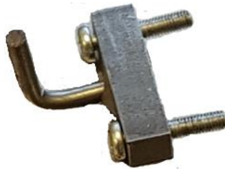
Figure 8: Shear Frame Hook
