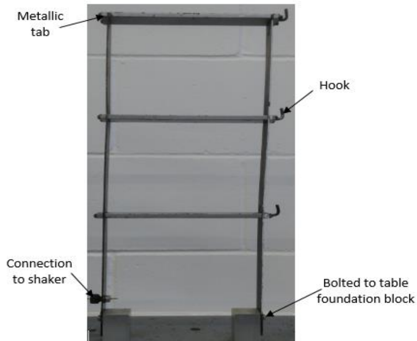
Figure 1: Photograph of the shear frame structure.
