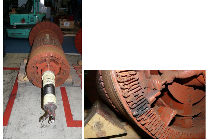
Fig. 5. Rotor winding short circuit causing the generator failure of wind turbine A103 in 01/2013.
