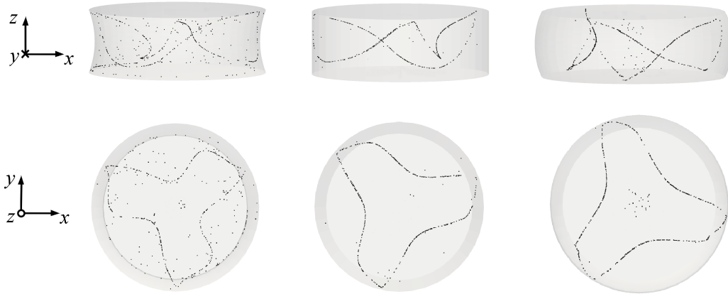
FIG. 10: Lateral and top views of PAS obtained numerically for the case AR = 0.34 and three different volume ratios: S = 0.92 ( t^* \approx 0.375 ) (left), S = 1 ( t^* \approx 2.5 ) (center), and S = 1.1 ( t^* \approx 0.88 ) (right). Flow conditions are summarized in Table IV. (For the axial views, the larger circle represents the periphery of the closest disk, while the smaller circle is the periphery of the opposite disk; the shaded region corresponds to the axial projection of the interface). The same perspective mode has also been used for other similar 3D figures included in the present work.
