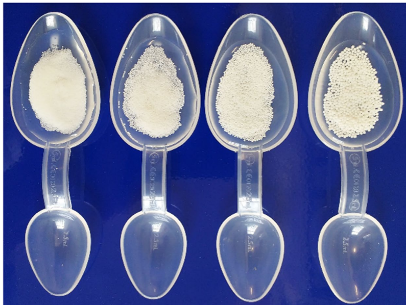
Figure 5. Samples of 500 mg of placebo multiparticulates dispersed in approximately 3 ml of spring water on a medicine dosing spoon. The particle size of the multiparticulates varies, from left to right: 200–355, 350–500, 500–710 and 700–1000 \mu\text{m} .
