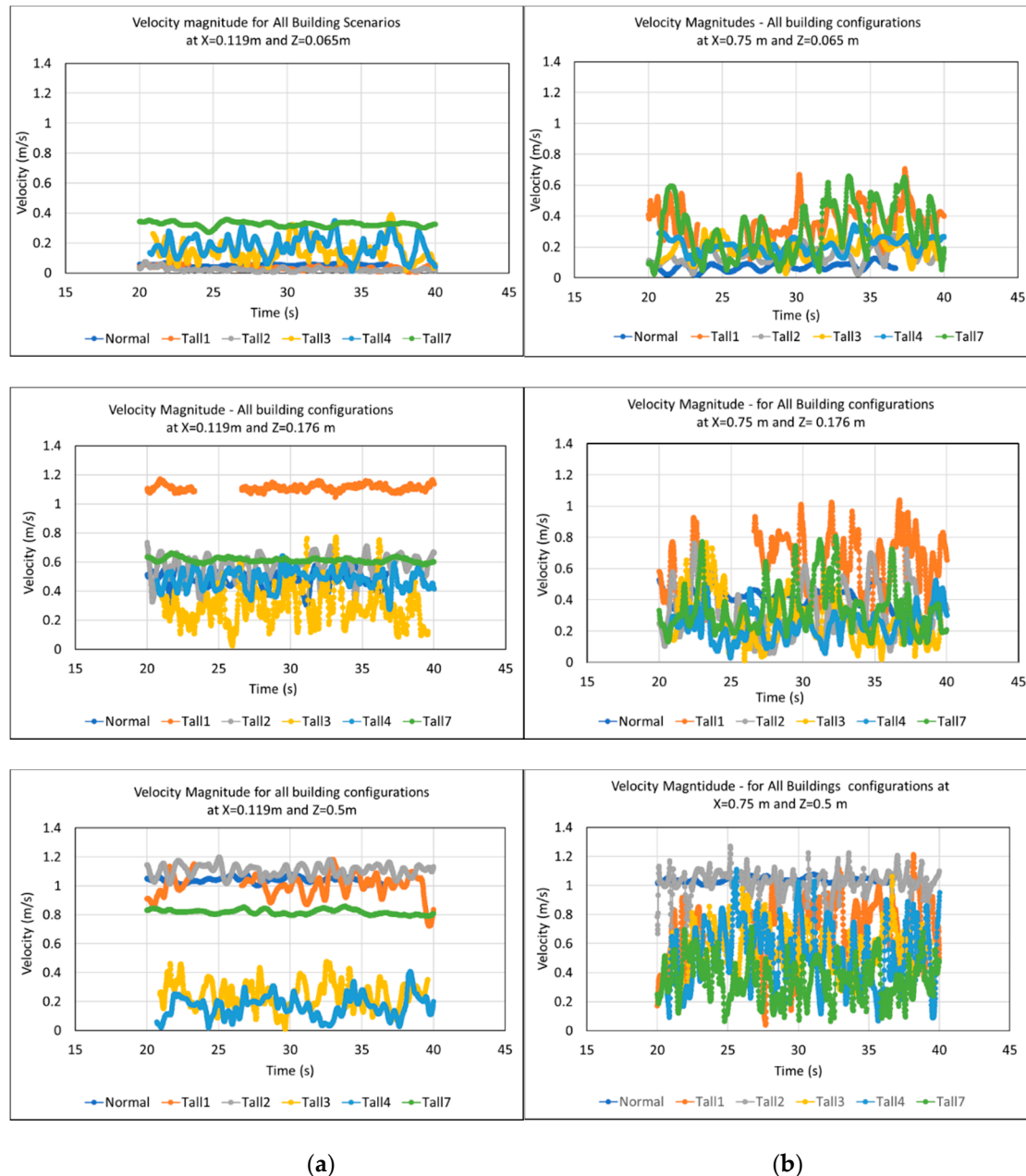
Figure 5. Variation of velocity magnitude at three different heights (a) within the building area ( X = 0.119 m, Y = 0.0 m) and (b) downstream the building area ( X = 0.75 m, Y = 0.0 m).
