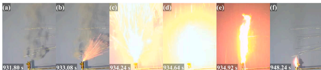
Fig. 2. Evolution from ignition to extinguishment of the cell with 100% SOC captured by the HD camera: (a) white smoke and gases, (b) sparks, (c) firework, (d) fireball, (e) jet fire, and (f) extinguishment.
