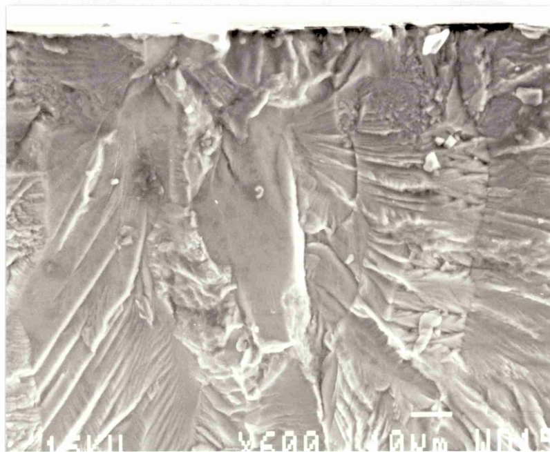
Figure 4.12 Fracture surface of alloy B, showing a faceted fracture feature associated with stage I growth.
