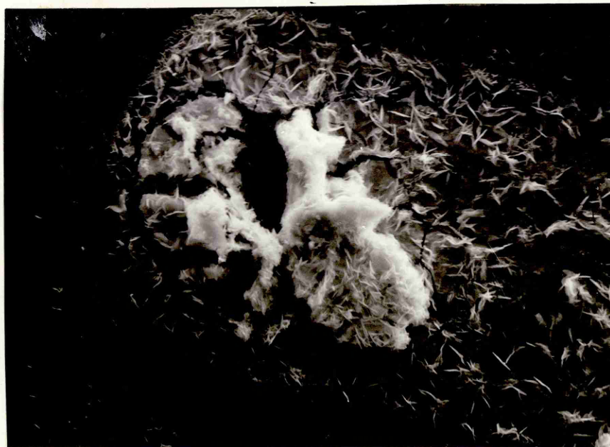
Figure 10 Photograph Of A Partially Covered Pit, Which Had Developed On Aluminium On Exposure To Lead Chloride Solution
