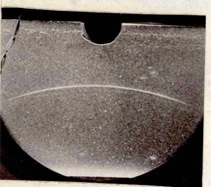
Fig. 4.18 Schlieren images of an ultrasonic pulse transmitted by a 25 mm radius cylindrical \text{PVF}_2 transducer, spreading out and being reflected from the bottom of the water tank. The water in the tank is approximately 200 mm deep.
