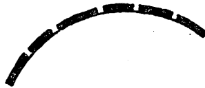
Fig. 11.2 Sectioned curved transmitting transducer. (Cross section)
