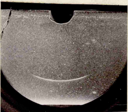
Fig. 4.18 Schlieren images of an ultrasonic pulse transmitted by a 25 mm radius cylindrical \text{PVF}_2 transducer, spreading out and being reflected from the bottom of the water tank. The water in the tank is approximately 200 mm deep.
