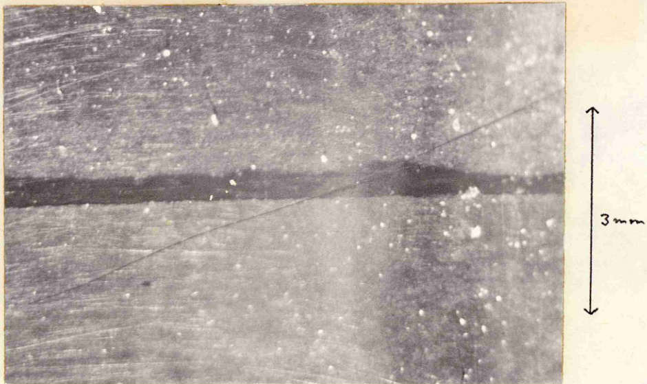
Fig. 4.23 Close up of damage to transducer. Diagonal line is a discontinuity in the gold coating on the active area of the \text{PVF}_2 foil.
