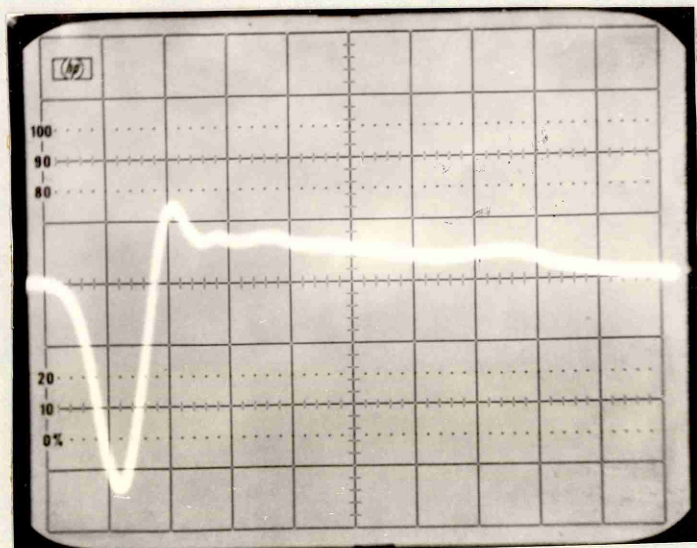
Fig. 4.27 Waveform received from 25 \mu\text{m} PVF 2 driven by pulse in fig. 4.26. 50 ns per division.
