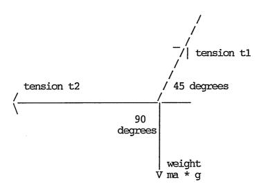
Without use of Lami's Theorem, one can find t2 in terms of ma and g by resolving vertically and horizontally:
