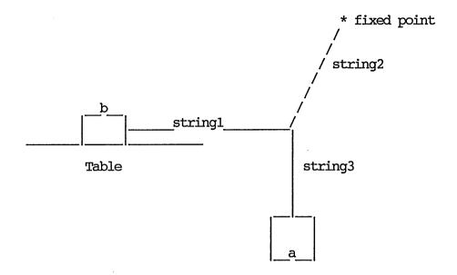
Problem: A block of mass mb rests on a rough horizontal plane, whose coefficient of friction is mu, the block being in limiting equilibrium. The block is pulled by a horizontal string attached to two other strings, one at an angle of 45 degrees to the horizontal whose other end is fixed, and one hanging vertically. On the other end of the vertical string a mass of ma is suspended. Find ma.
