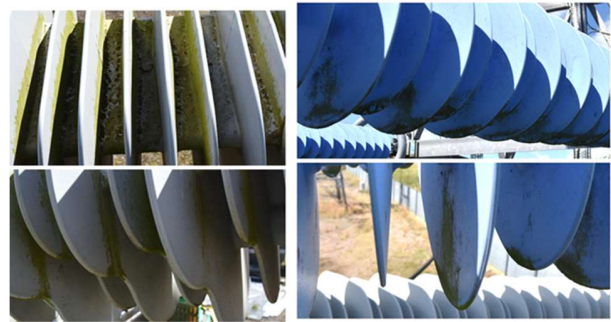
Figure 12. Biological growth after 56 months. Left: on top surface and on sheds of WC insulator. Right: on the WT insulators.
