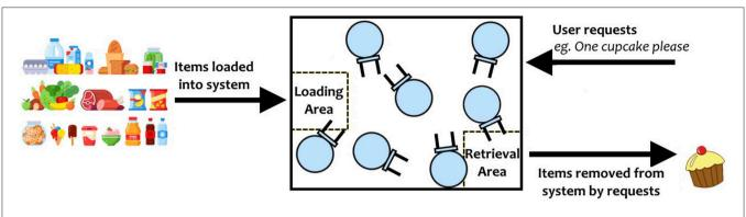
FIGURE 2 | The swarm system described to the interviewee. The storage organization system is described as automatically sorting stock input, and producing items upon user request. How the swarm operates within the box is not described.
