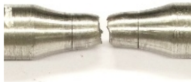
b) Fractured S355 coupon after test
