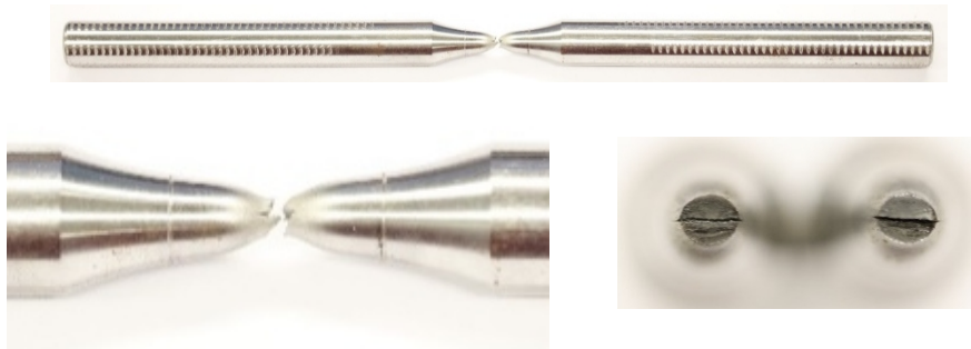
c) Fractured S690 coupon after test
