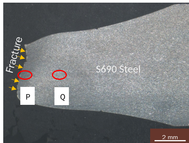
b) Longitudinal sectional view of the fractured coupon
