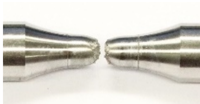
c) Fractured S690 coupon after test
