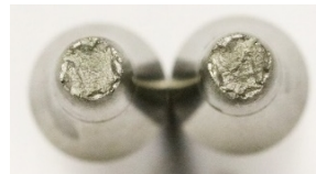
c) Fractured S690 coupon after test
