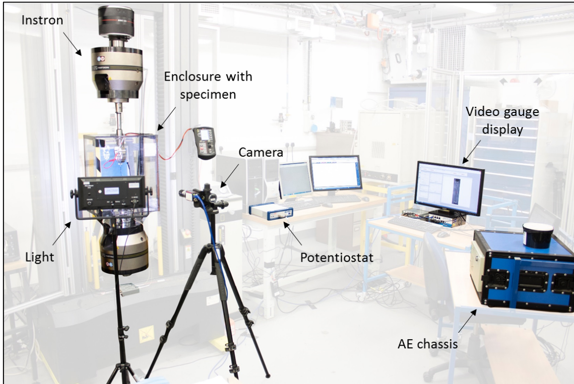
Fig. S11. Photograph of the bundle composite tensile test set-up with in-situ AE and electrical conductivity measurement. The video gauge camera and associated software records the pixel displacement from two painted marks on the sample surface. The sample is illuminated using a light source to ensure a suitable contrast for the video gauge software to track the points accurately. The force and displacement outputs from the Instron were also recorded in-situ with the strain measurements to ensure simultaneous data acquisition via an analogue to digital converter. In conjunction with these recordings acoustic emission events were detected through sensors placed on the sample's surface and processed by the AE chassis and associated software. Similarly, a fixed voltage was applied to the sample, in the loading direction, and the current recorded using a potentiostat to evaluate strain-dependent resistivity.
