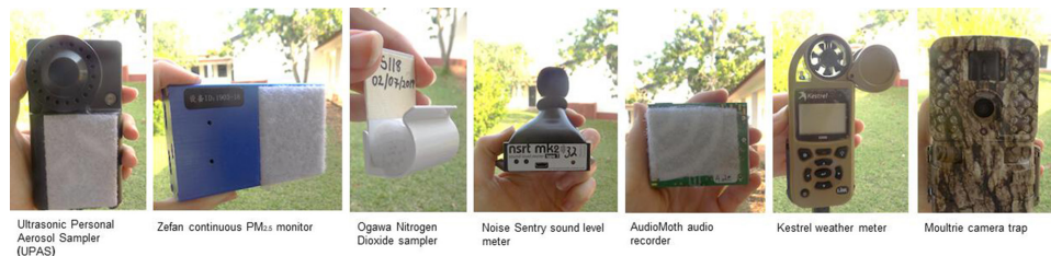
Figure 3 Images of environmental monitoring equipment.
