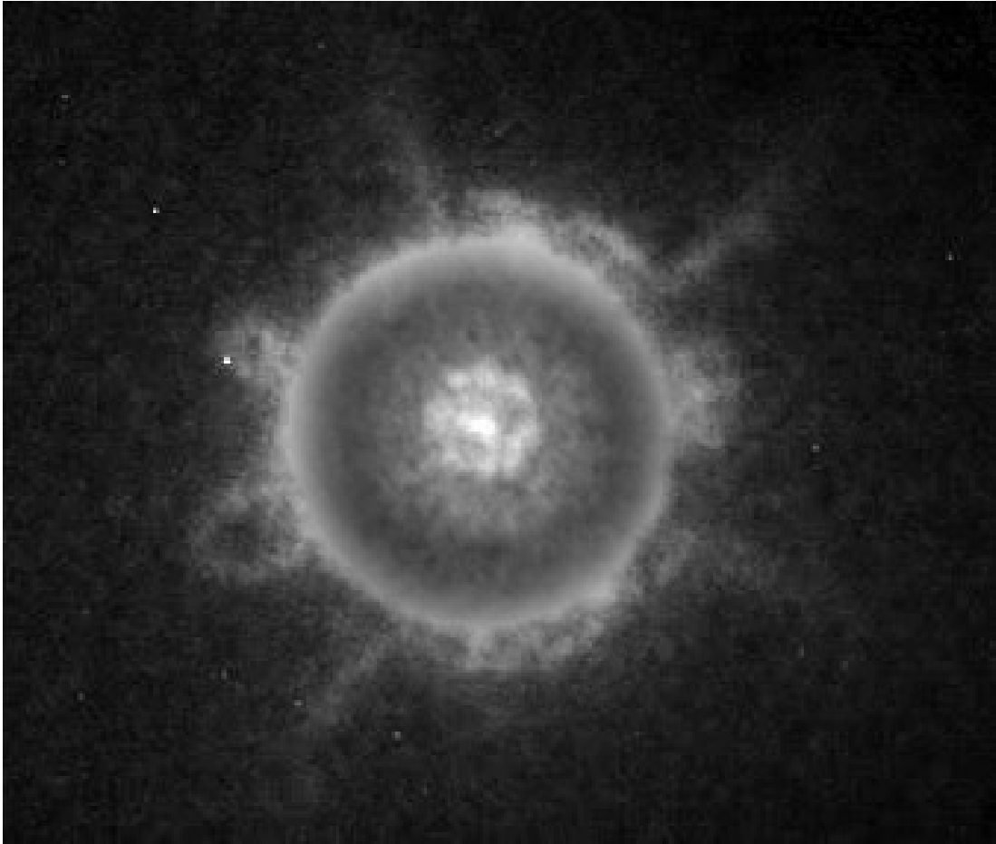
Figure 3.3: End-on captures of the visible emission from the plasma occasionally show what appear to be loops. (Image has been modified to enhance clarity of outer region.)
