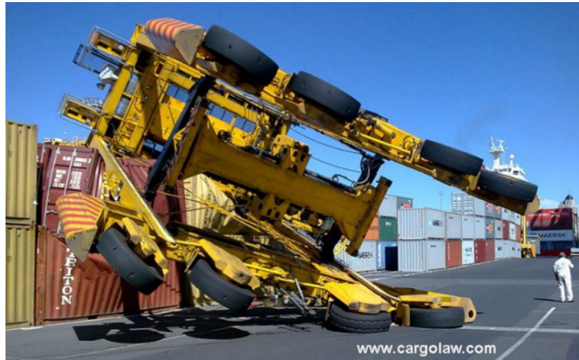
Figure 2-6. Toppled straddle carrier. Source: Cargolaw 2
