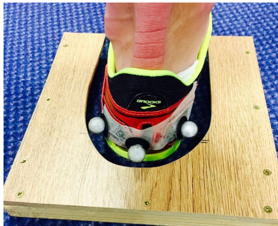
Figure 4.2.2.2 Custom built block to enable consistent placement of calcaneus markers
