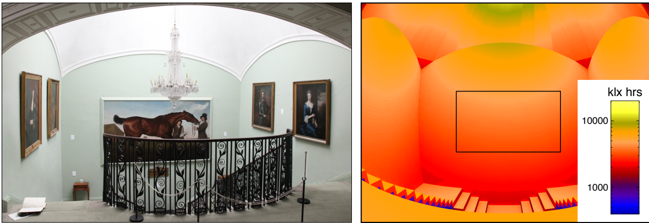
Figure 2: Photograph showing Hambletonian displayed on the Stone Staircase at Mount Stewart (Belfast, Northern Ireland) alongside CBDM simulation of cumulative annual illuminance (available in colour in online version)
