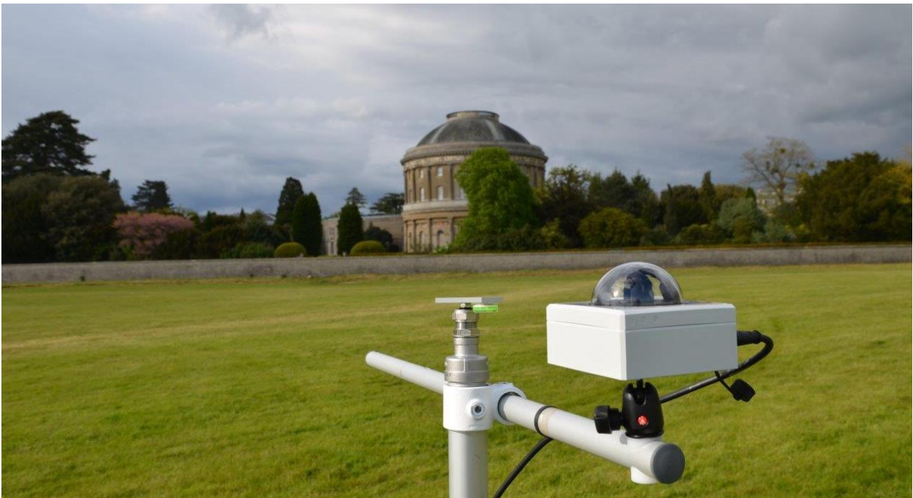
Figure 8: Delta-T BF5 sunshine sensor in the grounds at Ickworth House (available in colour in online version)
