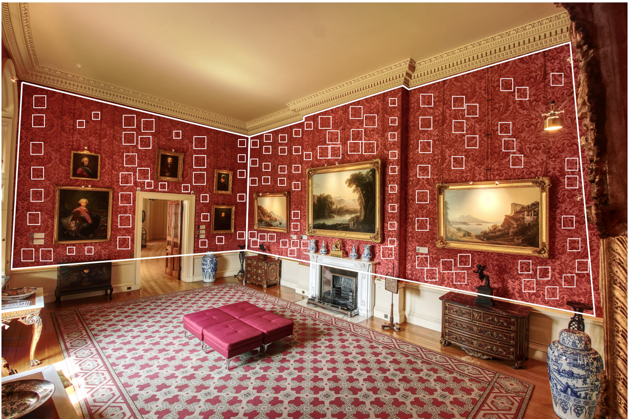
Figure 6: Image of the Smoking Room showing the wallpaper patches used for the interpolation of the illuminance map (available in colour in online version)
