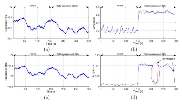
Figure 4.7 The analysis of the characteristic frequencies in the current signal using the IDFT under variable speed conditions (a)  $C_1$  (b) Its amplitude over time (c)  $C_2$  (d) Its amplitude over time.
