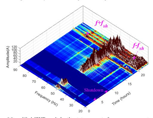
Figure 6.9 modified CWT result for the stator current after an emergency stop on  $4^{th}$  April 2016.
