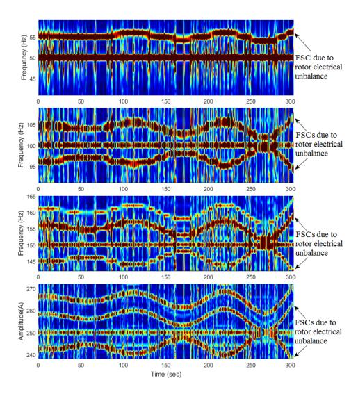
Figure 6.3 Modified CWT result for the current signal when the rotor electrical unbalance was simulated at variable rotational speed.
