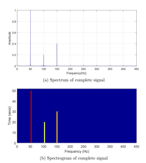
Figure 4.2 Analysis of a non-stationary signal via the (a) FFT and (b) STFT.
