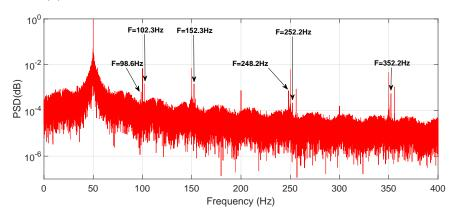
(b) Simulated data under 23% of rotor electrical unbalance
