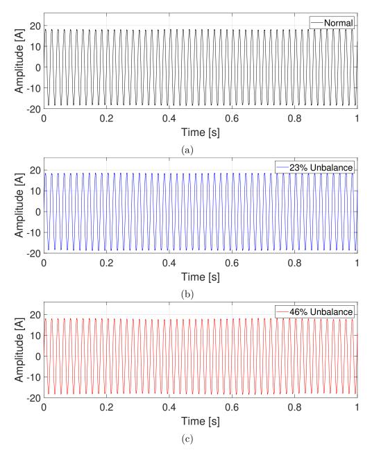
Figure 5.2 Comparison of the current-time waveform for healthy case, 23% rotor unbalance case and 46% rotor unbalance case.
