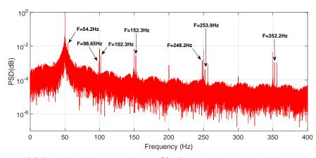
(c) Simulated data under 73.6% of rotor electrical unbalance
