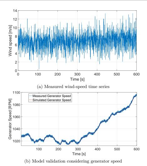
Figure 3.11 Actual variable speed driving conditions.
