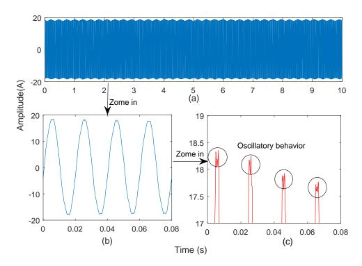
Figure 6.1 The generator current signal (a) during 10sec, (b) zoomed between 0 and 0.08sec and (c) zoomed for the positive peaks.
