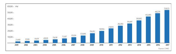
Figure 1.2 Global annual cumulative wind capacity 2001-2017 according to [1].
