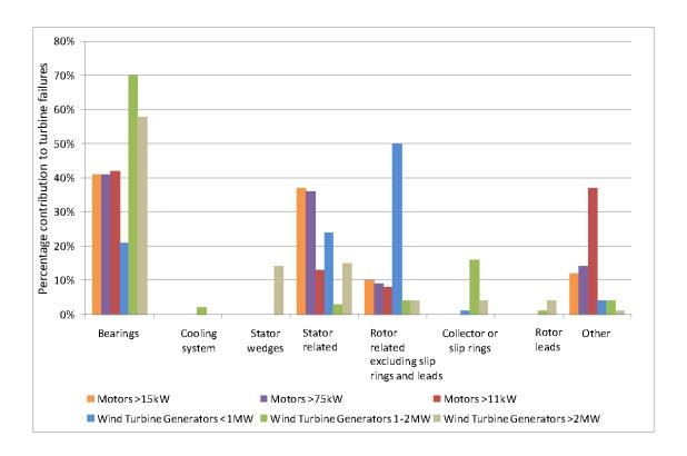
Figure 2.3 Comparison of failure contribution of WT generator components according to [3, 4].
