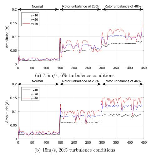
Figure 6.8 Tracking the magnitude of fault signature frequencies of interest for the detection of rotor unbalance.
