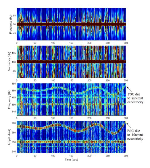
Figure 6.2 Modified CWT results when tracking the current signal with an inherent eccentricity simulated at variable rotational speed.
