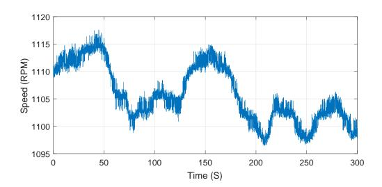
Figure 4.5 Generator speed for analysis using the IDFT algorithm.
