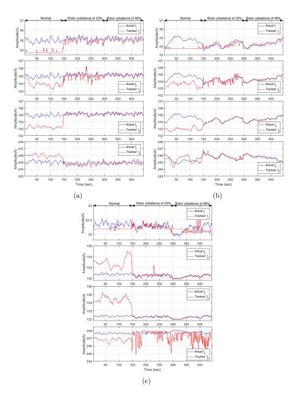
Figure 5.14 Tracking the fault frequencies of interest using EKF for (a) test case 1 (b) test case 2 and (c) test case 3.
