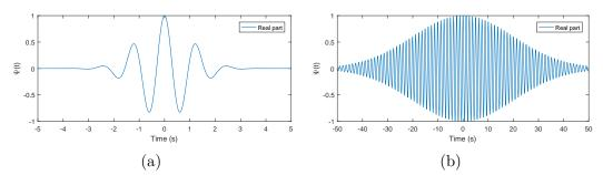
Figure 6.4 Mother wavelets with different values of the parameter  $\sigma$  (a)  $\sigma = 1$  and (b)  $\sigma > 1$ .
