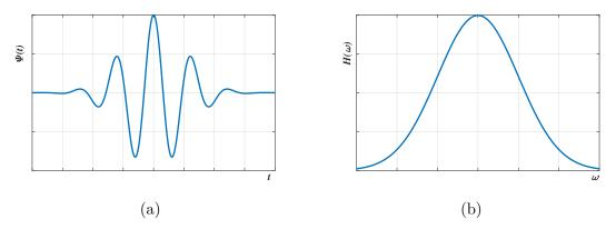
Figure 4.3 (a) Morlet wavelet in time domain and (b) frequency domain.
