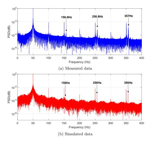
Figure 3.8 Normalized stator current spectra with inherent static eccentricity.
