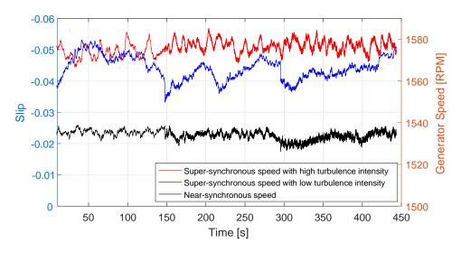
Figure 5.4 Generator speed test conditions.
