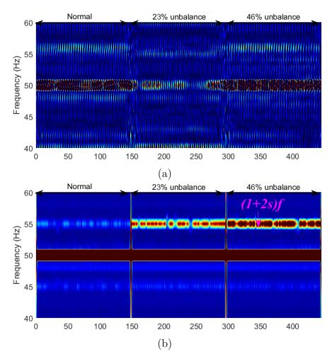
Figure 6.6 Time frequency representation of the current signal using the (a) conventional CWT and (b)modified CWT with the test rig driven by 15 m/s, 20% turbulence conditions.
