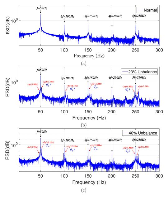
Figure 5.3 Comparison of the current spectra for healthy case, 23% rotor unbalance case and 46% rotor unbalance case.
