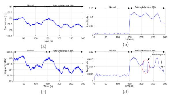
Figure 4.8 The analysis of the characteristic frequencies in the current signal using the IDFT under variable speed conditions (a)  $C_3$  (b) Its amplitude over time (c)  $C_4$  (d) Its amplitude over time.
