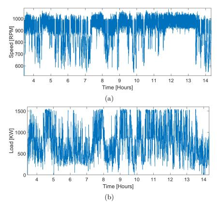
Figure 3.10 Operational data from a 2.5 MW variable speed WT (a) Generator speed and (b) Load.
