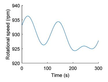
Figure 4.11 Rotational speed variation in simulation study.
