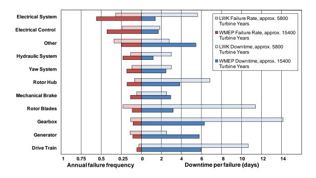
Figure 2.2 Failure frequencies of major WT subsystems and downtime caused by failures of these subsystems [2].
