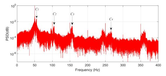
Figure 4.6 Simulated stator current spectra with inherent static eccentricity and rotor electrical unbalance at variable speed conditions.
