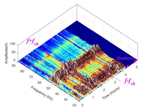
Figure 6.10 modified CWT result for the stator current before an emergency stop on  $5^{th}$  April 2016.
