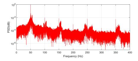
Figure 3.12 Simulated stator current spectra with inherent static eccentricity and rotor electrical unbalance at variable speed conditions.
