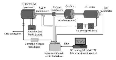
Figure 5.1 Schematic representation of the test rig[5].
