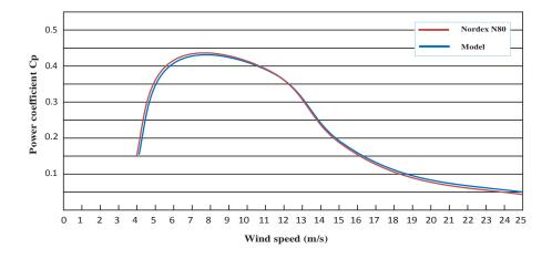
Figure 3.3 Comparison of the numerical approximation of the power curve with the power curve of the commercial Nordex N80-2.5MW wind turbine.
