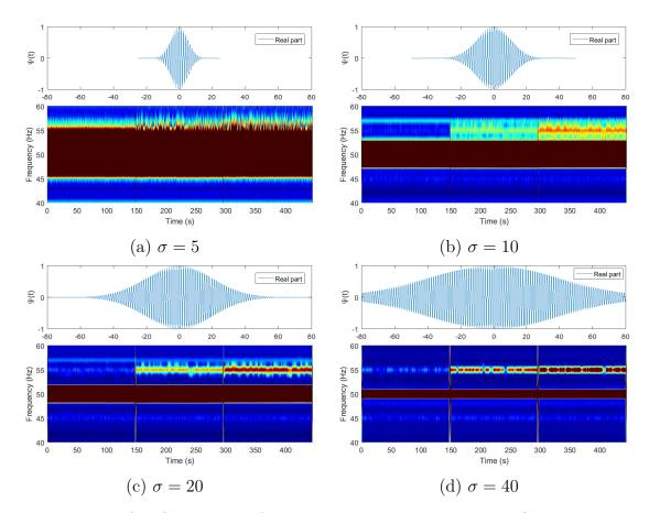
Figure 6.7 modified CWT results for the current signal using various Gabor wavelets
