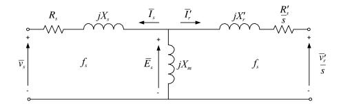
Figure 3.6 DFIG equivalent electric circuit referred to the stator.
