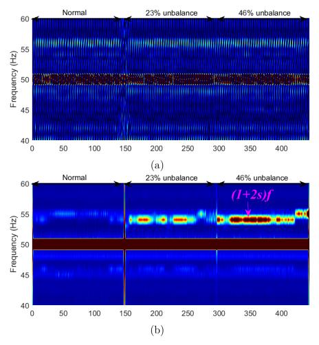
Figure 6.5 Time frequency representation of the current signal using the (a) conventional CWT and (b)modified CWT with the test rig driven by 7.5 m/s, 6% turbulence conditions.
