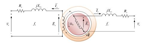
Figure 3.5 DFIG equivalent electric circuit with different stator and rotor frequencies.
