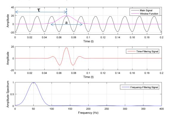
Figure 4.1 Graphical illustration of the STFT for extracting the time-frequency content of a measured signal.
