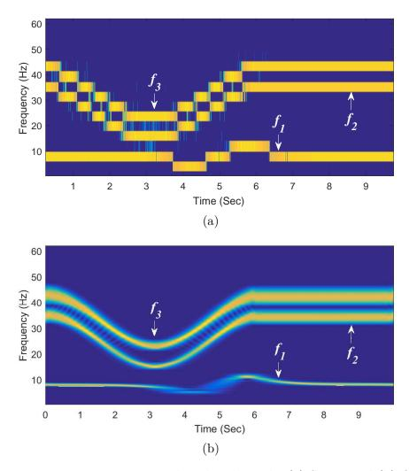
Figure 4.4 Non-stationary signal analysed via the (a) STFT and (b) CWT.
