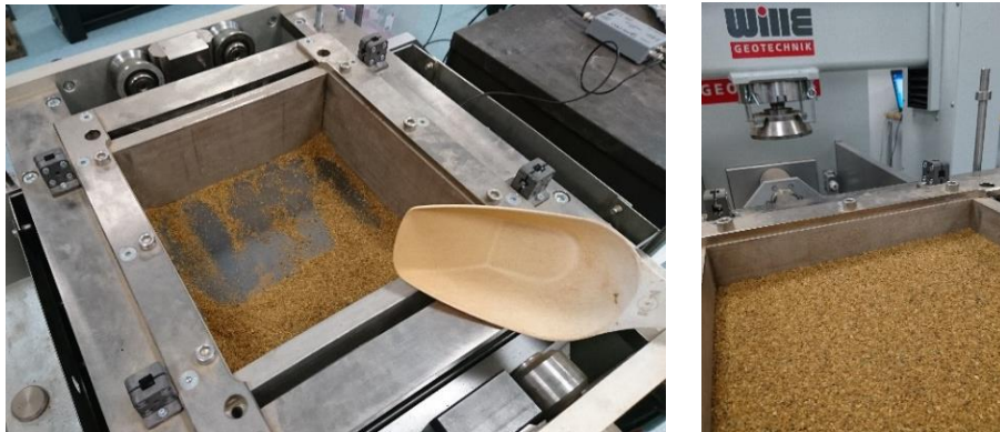
Figure 3.28 Filling the top box of the shear box with soil.
