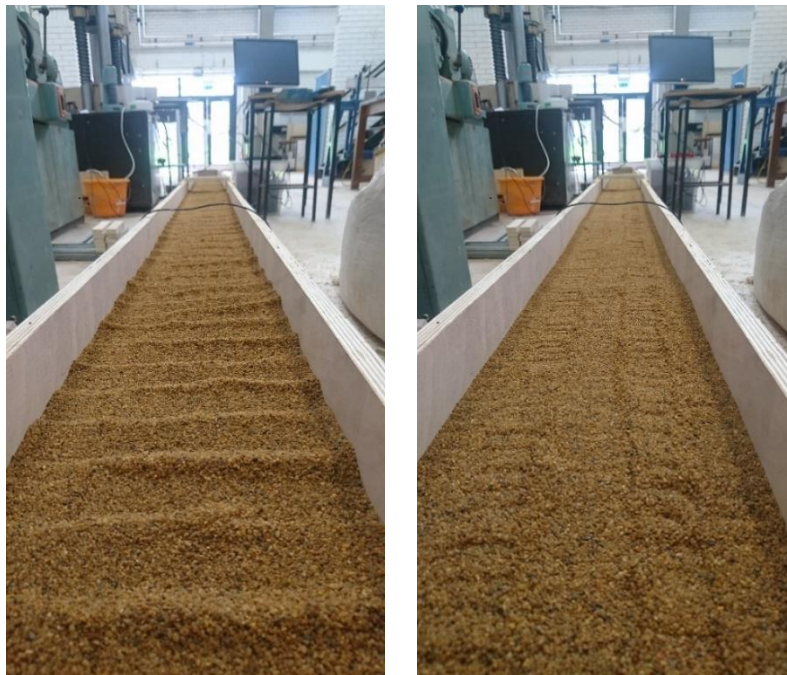
Figure 3.38 Photographs of the systematic densification process during set-up of large-scale tests.
