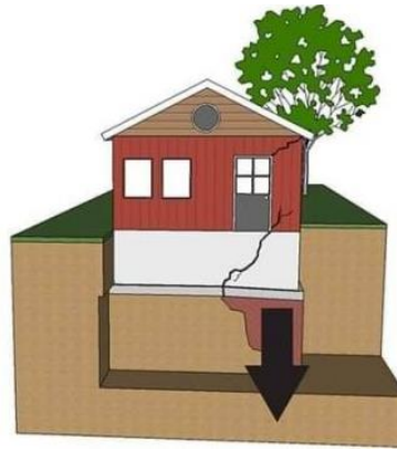
Figure 2.3 Cracking caused by the differential settlement of a building. Adapted from Geotech (n.d).
