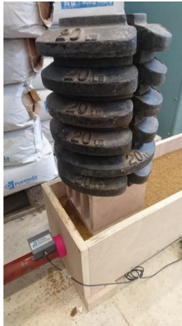
Figure 3.39 Weight towers constructed on a block and used to apply a normal stress and force soil-steel interactions in large-scale laboratory experimentation.
