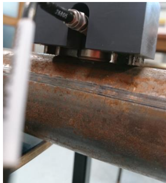
Figure 2.27 A butt-welded pipe with welded seam.
