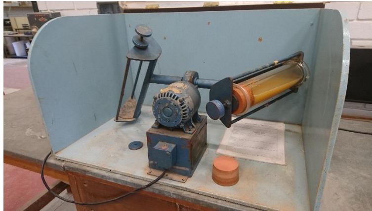
Figure 3.23 Over-end turning process during a bell jar test to characterise soil density.
