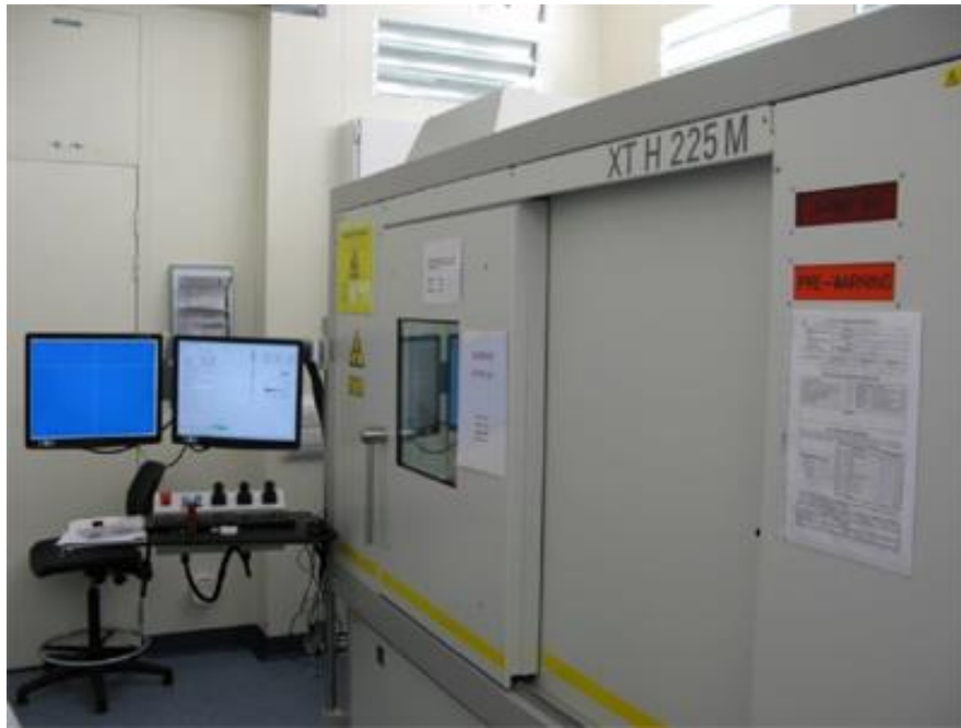
Figure 50. Photograph of MCT225 system at the National Physical Laboratory (NPL), Teddington. Image courtesy of NPL.
