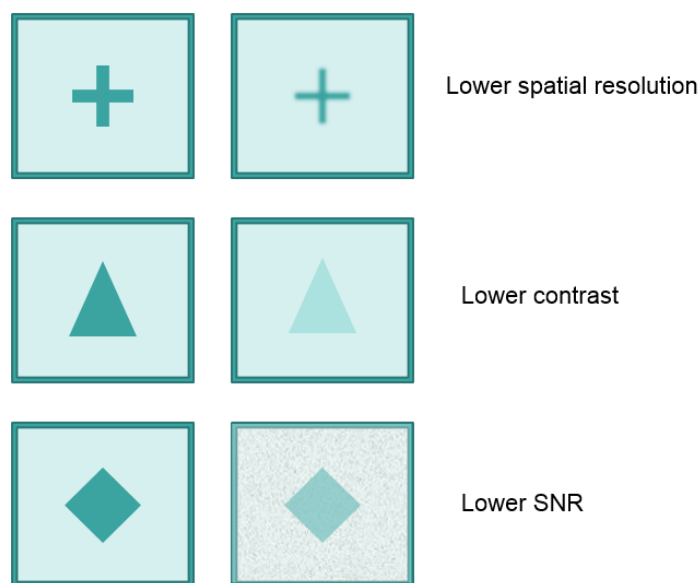
Figure 15. Schematic of image quality parameters, spatial resolution, contrast and noise. An example of the influence of these qualities on the resulting image is demonstrated.
