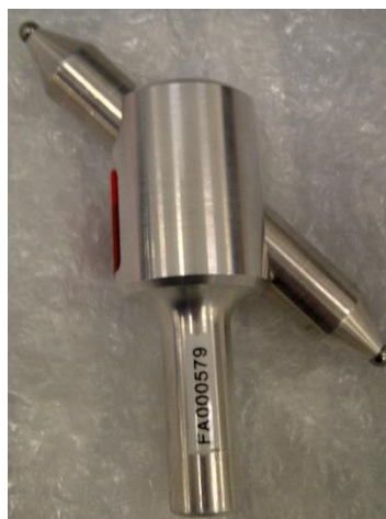
Figure 42. Image of CT ball bar. Steel balls fixed to ends are located with tactile CMM to create a calibrated reference length. The ball bar is scanned by the CT system and used to scale the dataset.
