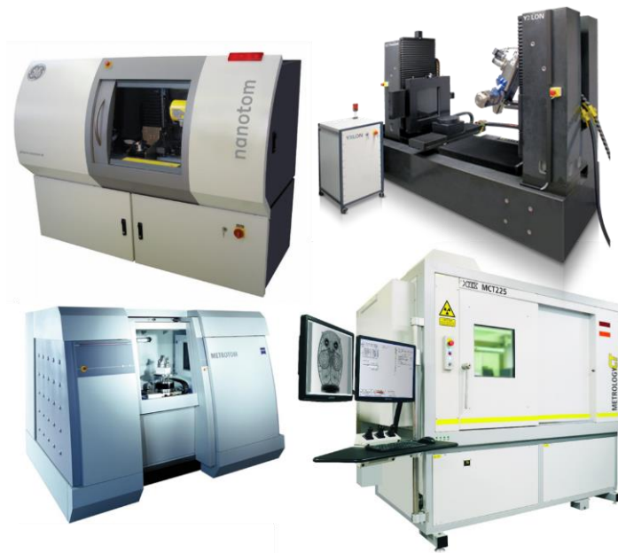
Figure 5. Example of a Metrology CT systems by a number of manufacturers. Clockwise from top left: Nanotom from GE [31], CT-Precision from YXLON [32], Metrotom from Carl Zeiss [33] and MCT 225 from Nikon Metrology [34].
