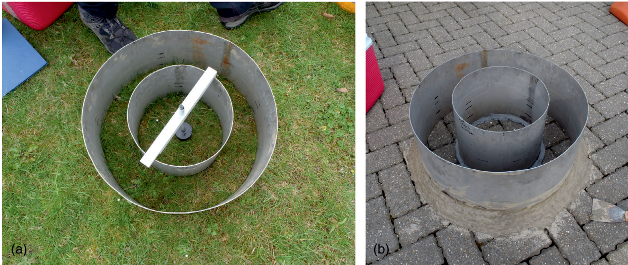
FIGURE 4 Infiltrometer installed in the a) Green Area and b) the permeable pavement area
