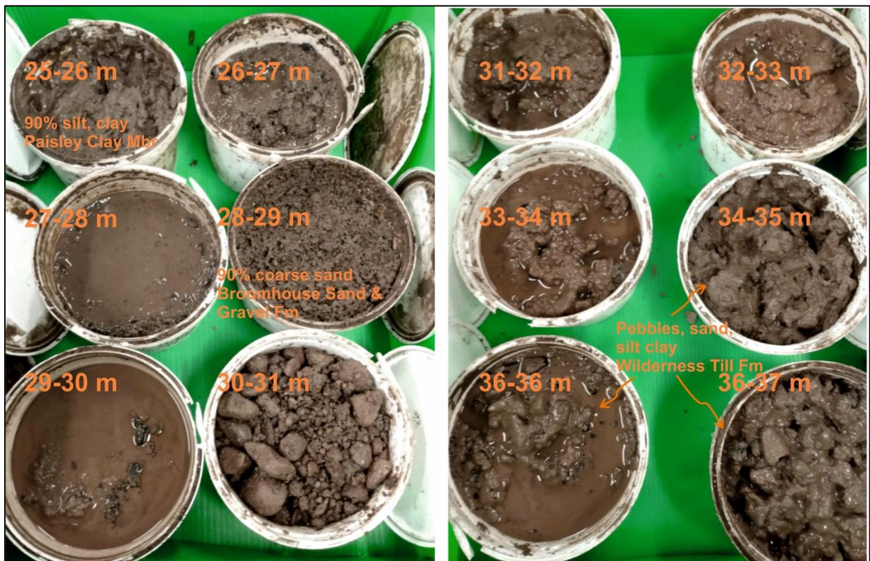
Figure 5 Image of the superficial deposits returned for GGA05 from 25 – 37 m drilled depth
