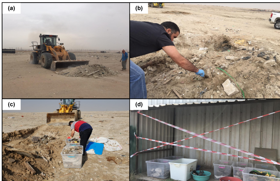
Fig. 1. Pictorial Analysis of Sampling Procedure Followed For Waste Reclamation Using (a) Spade Tractor to Excavate The Landfill Ditch; (b) Obtaining Black Matter Where Waste is Buried; (c) Reclaiming The Waste, and (d) Segregating The Material Before Washing. Published with permission from. Source Al-Salem et al. [34] (Published with permission)
