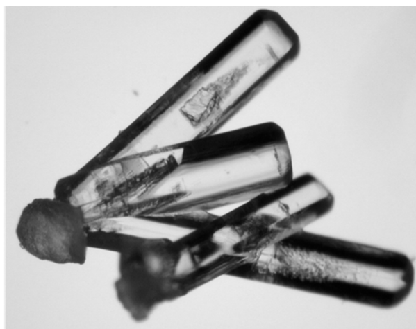
Figure 1.12: Form II, the metastable orthorhombic polymorph of acetaminophen growing from isotactic polypropylene beads. Reproduced from reference 147 with permission. Copyright 2002, American Chemical Society.
