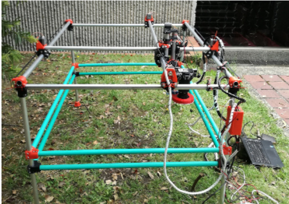
Fig. 3. Improvised land mine detection platform in action. For testing purposes, the test terrain is scanned via a Cartesian robot.
