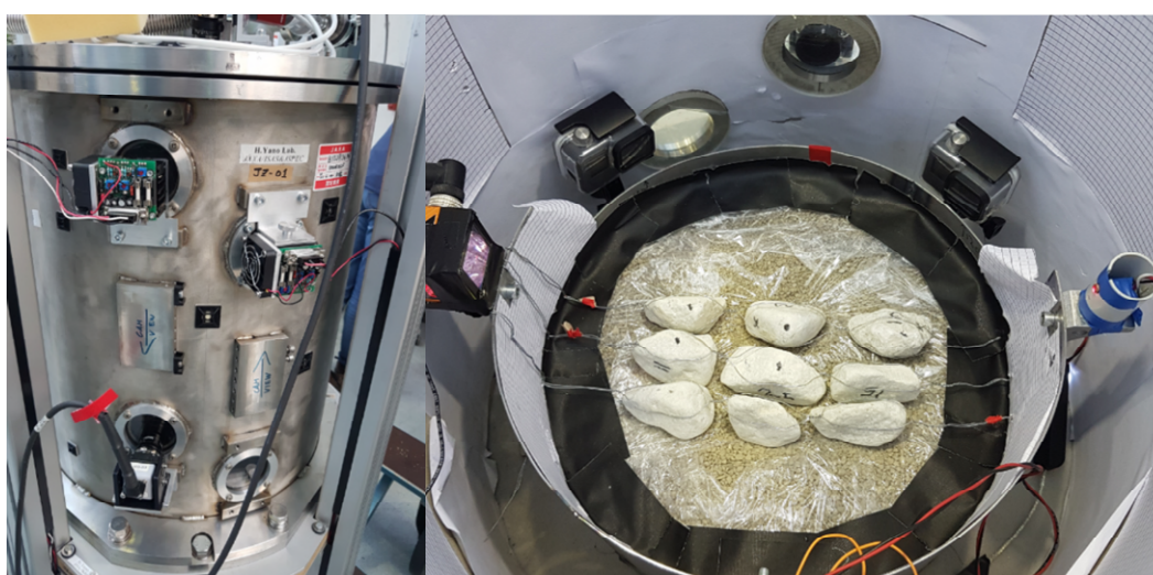
Figure 6. Sensors Setup. The external view (left) shows the bottom FC camera and two lamps attached to windows on the side of the vacuum chamber. The interior view (right) shows the two GoPros, separated by 90°, with the FC camera seen from the middle window. The light gate is seen attached at the top of the container, with the receptor (right side in blue) diametrically opposed to the emitter.
