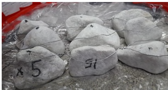
Figure 11. Surface analogue Final Set-up. Addition of rocks on top of ESA03A – KM Bentonite
