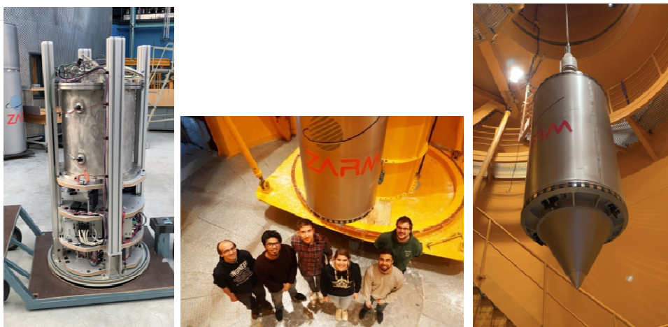
Figure 3. (Left) Experiment setup inside JAXA's vacuum chamber, mounted inside open ZARM Capsule. (Centre) Land3U team. (Right) ZARM Capsule being winched up to the top of the tower.
