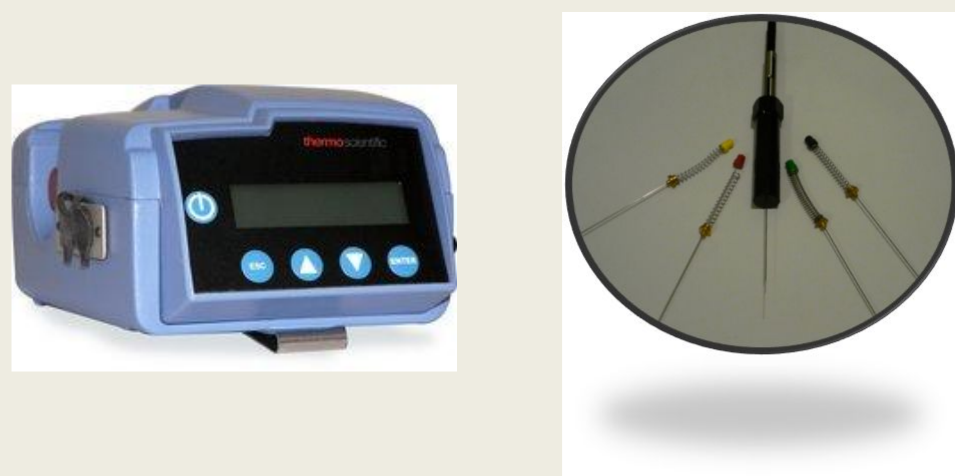
Figure 1: Left picture is the particulate matter monitoring instrument and the right picture is the SPME holder and fiber options.
