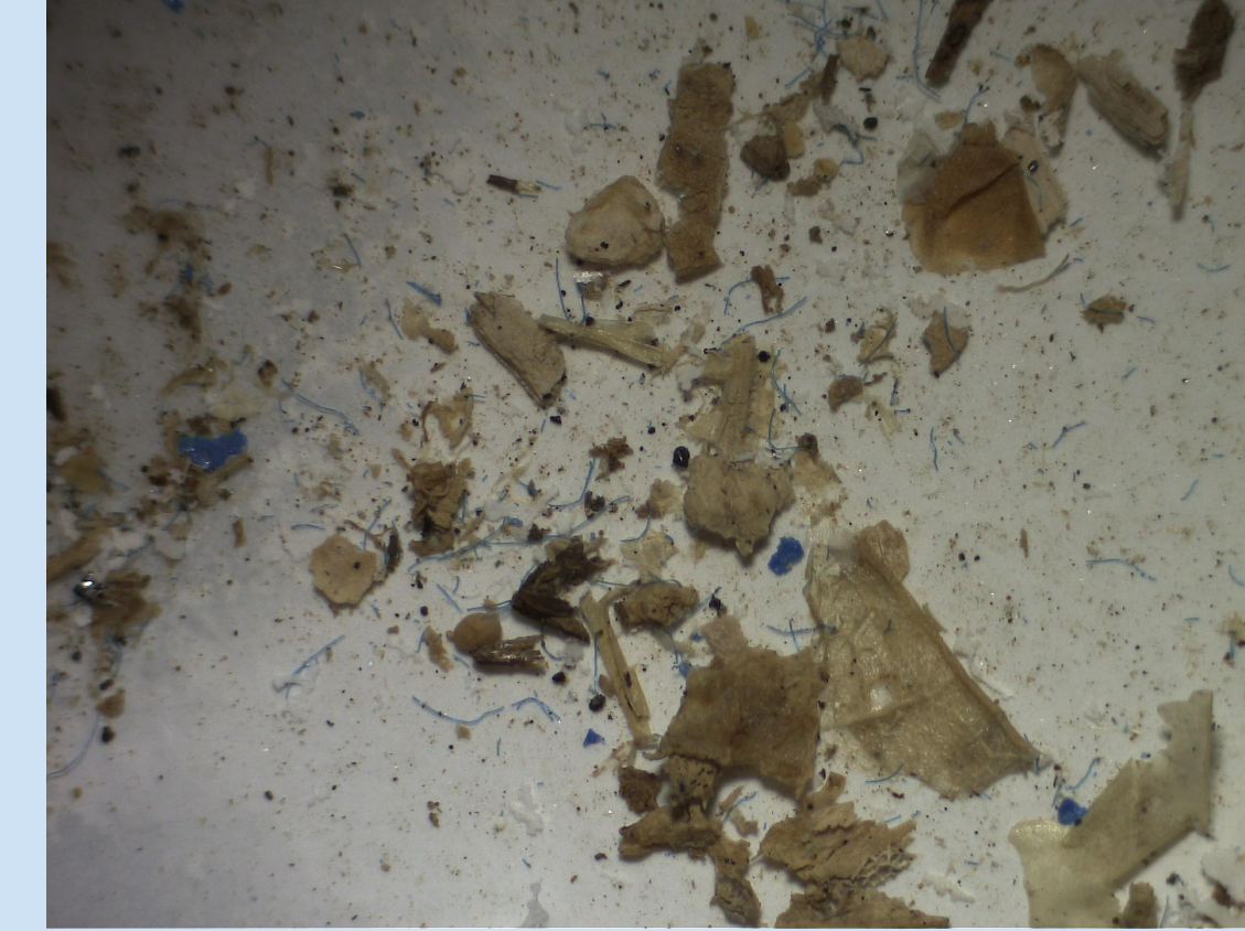
Figure 5: Microfibers under stereomicroscope at 10x.
