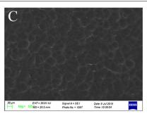
FIGURE 2 | SEM images of polyethylene-coated parchment (designated as A), polyethylene-coated nylon (designated as B), and greaseproof paper (designated as C). In (A,C), package materials the presence of fibers and micro-pores is evident. By contrast, B package material showed a smooth, plane, and homogeneous surface without holes or micro-pores able to entrap microorganisms.
