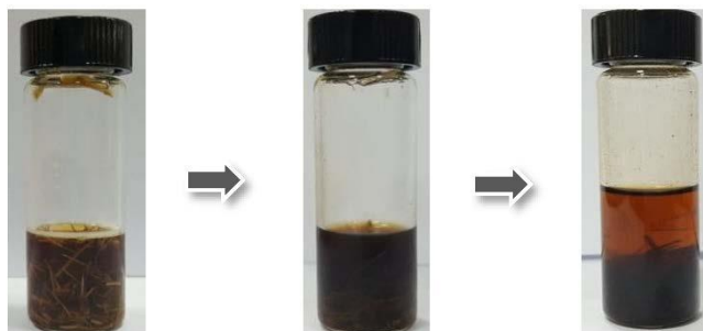
Figure 4. Biomass processing with CP 1:1 at different stages (From left: Before stirring, after overnight treatment, after centrifuging with ethanol).
