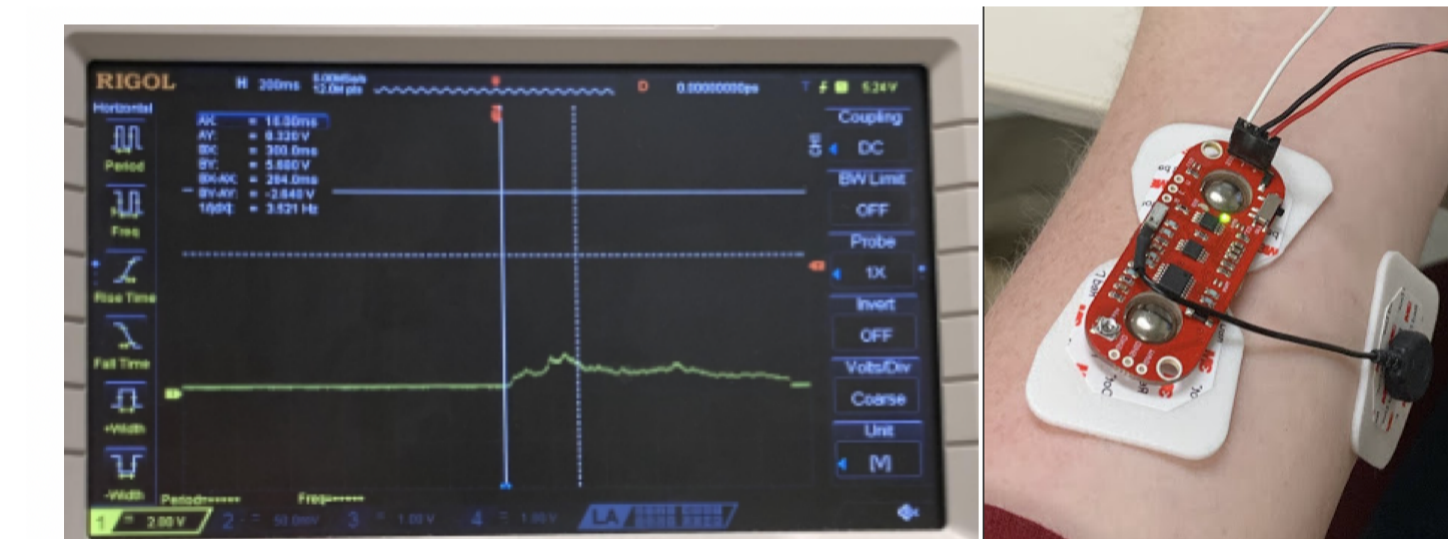
Figure 2: Example EMG wave and electrode placement
