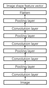
Figure 4. The CNN for extracting image shape feature
