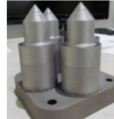
Figure 5a. Printed injection moulding inserts
