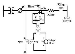
Figure 3 Line Drop Compensation Circuit
