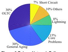
Figure 2 Eskom Network Failure Statistic of Transformers 20-100 MVA
