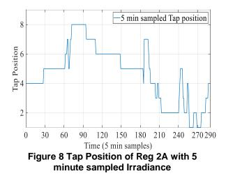
The annual of tap operations for different temporal resolutions of the solar irradiance incident on the panels is given in Table 2. From the numbers in Table 2 there is a significant difference between the number of tap operations registered in case of 1 minute sampled solar irradiance as opposed to the 5 minute sampled or a 1 hour sampled TMY3 data. However, the difference between the 5 minute sampled data and the TMY3 data is not so significant.
