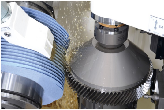
Figure 1. Tool (left) and part (right) in generating grinding [8]
