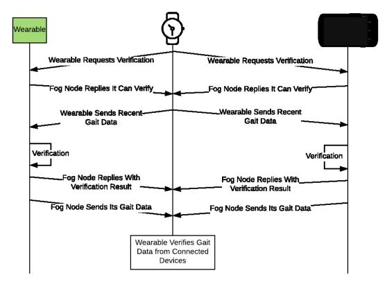
Figure 2. Communication Flow for Gait Verification
