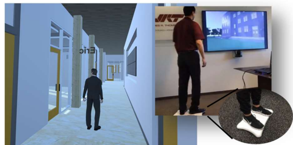
Fig.4 Test subjects are also asked to search for a person. We programmed Wii Balance Board for avatar control by leaning and walking on the board.
