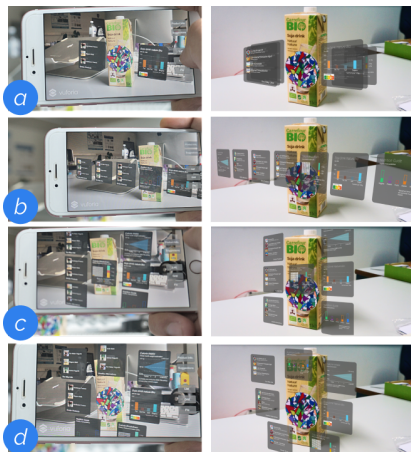
Figure 3. Different PHARA layouts. Left: Handheld. Right: HMD. a) stack, b) list c) grid and d) pie
