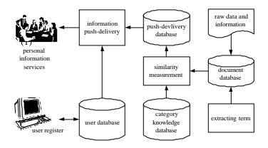
Figure 1. Architecture of personal information push-delivery system
