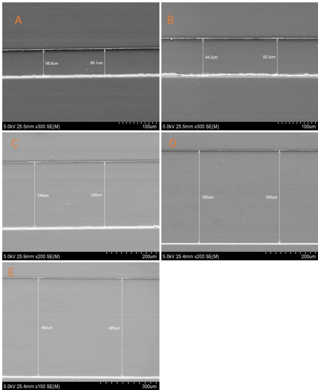
Figure 9. 14: SEM images of the linear channel widths from 75-500 μm (A-E) on Si wafers
