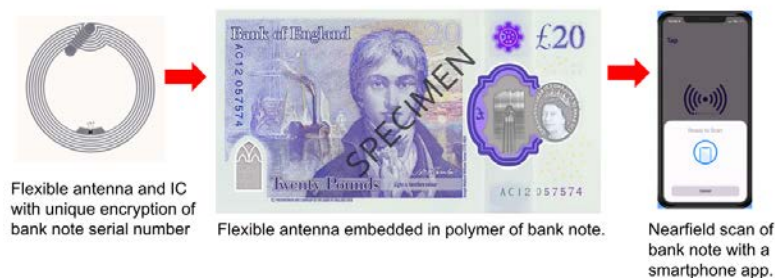
Figure 6. Schematic illustration of the application to a bank note of a flexible IC with a unique ID number (encryption cipher/key) maintained on a non-programmable coprocessor with a ROM.
