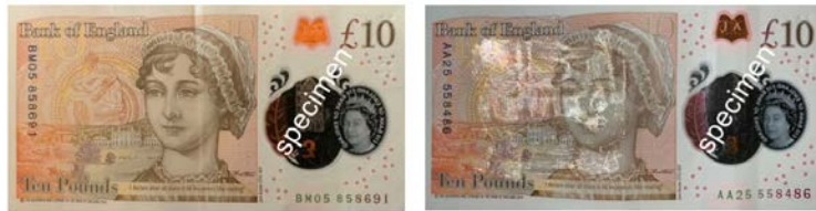
Figure 10. Smartphone images of a banknote with reflective powder applied under ambient lighting conditions (left) and with a LED halogen flash (right). The reflective power, consisting of a randomized complex of micro retro-reflectors, has been applied by doping a clear nail varnish with the powder and 'painting' it onto a rectangular patch that covers the central component of the notes principal graphic as shown on the example on the right-hand-side.
