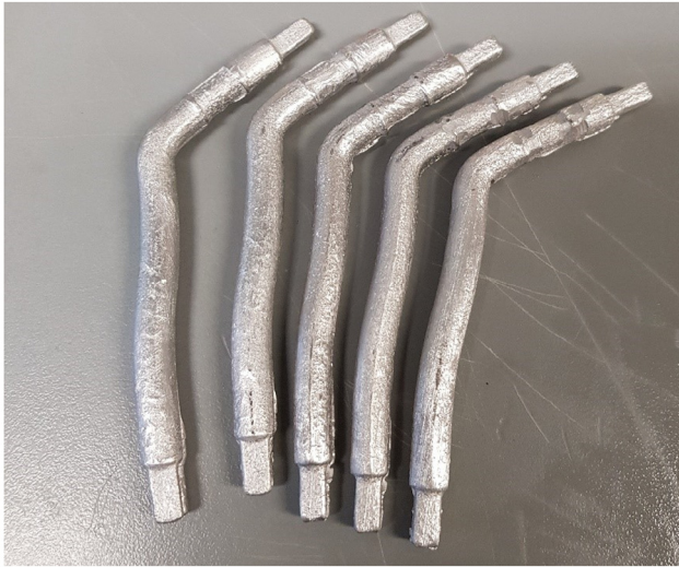
Fig. 1. Photographs of some lumen moulds made using the low melting temperature alloy material.
