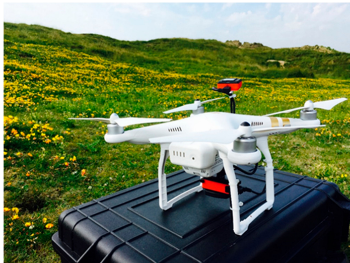
Figure 5. Sequoia multispectral sensor mounted on a DJI Phantom 3 Pro UAS. Photo taken by the author.
