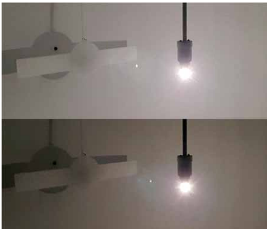
This image illustrates what a drop in output looks like for a bulb. The flux of the bottom image is 70% that of the top. This bottom case would mean the unit has reached the end of its useful life.
