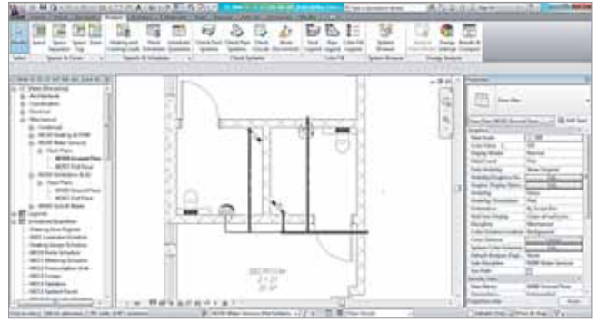
Figure 7: Automatically generating pipework layout.
